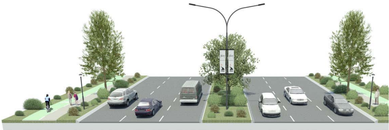
Figure 12: NMT Facilities along Kerbed Arterials (80km/hr and above), NDoT: NMT Facility Guidelines (2015: 58)
